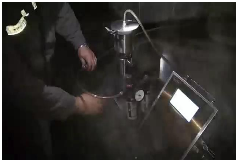
CWH12型瓦斯含量井下一站式自动化测定仪
