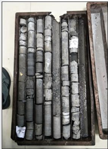
60m范围内顶板钻孔取芯
